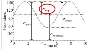
Folkman Equation:  $N_{cycles to failure}$ =  $10^{-4.196 \log(\sigma_{amp})+17.76}$
