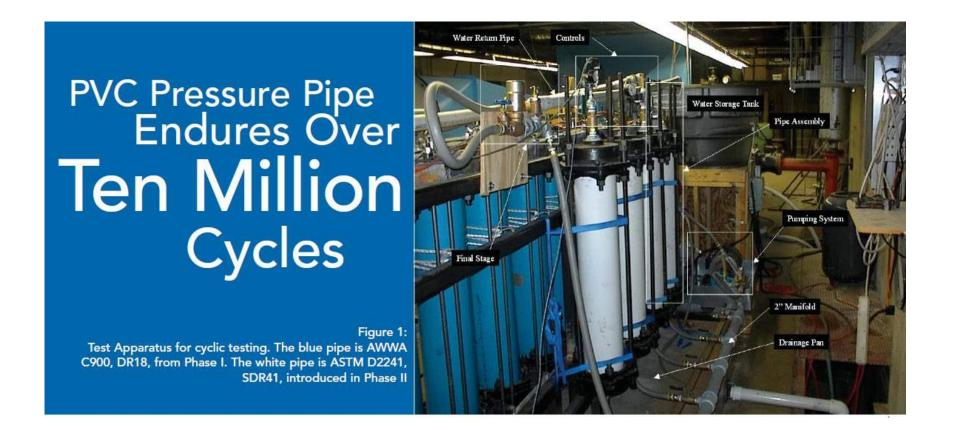
Cyclic testing of PVC pipe included pipe that reached over 10 million cycles and never failed
