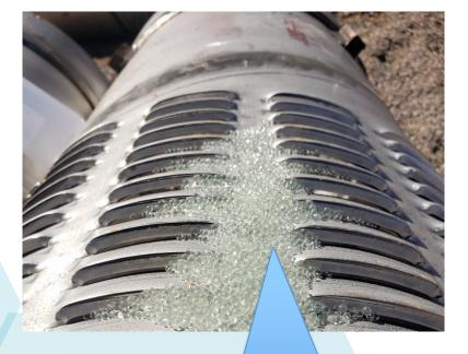
Advancements: Stainless Steel Well Screen & Glass Beads As A Filter Pack Media (Improved Hydraulics) What's Unique About Injection Wells?
